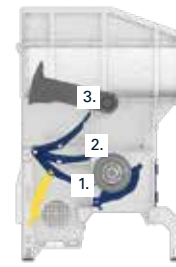
Hydraulic door for maintenance and removal of foreign objects
